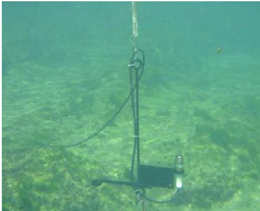
Figure 3. Underwater LI COR sensor used to measure PAR
