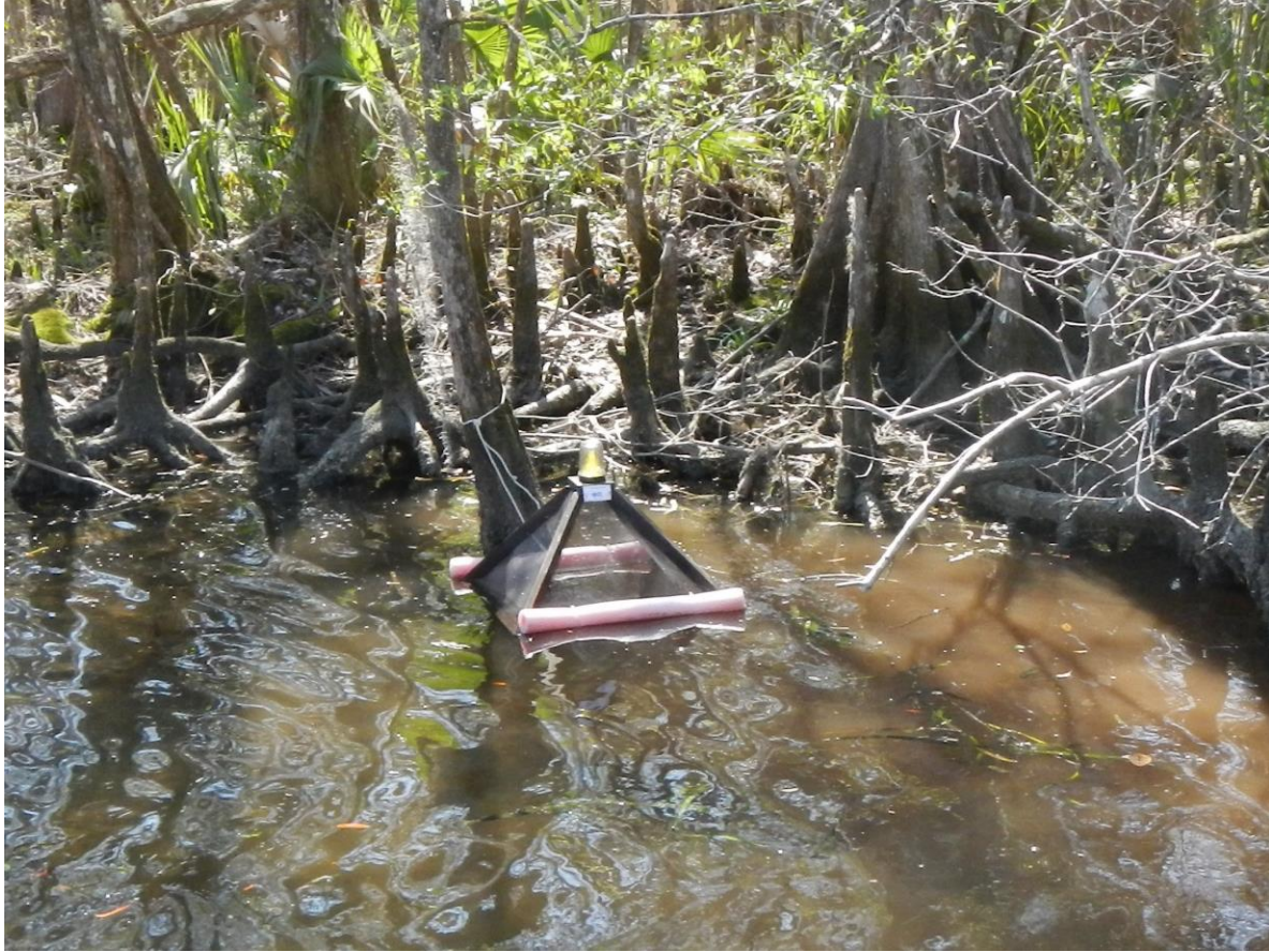
Figure 6. Trap used to collect adult aquatic insects as they emerge from the water
