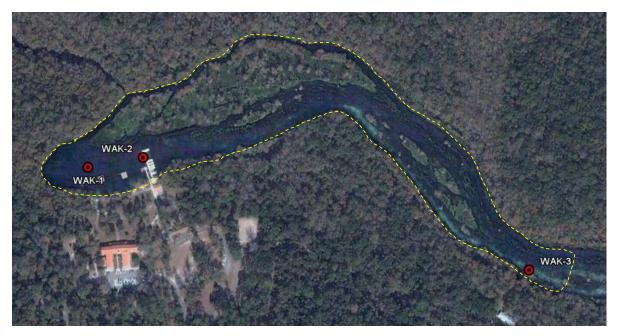
FIGURE 10 Illustration of the general area studied at Wakulla Springs (with data sonde locations as red icons).
